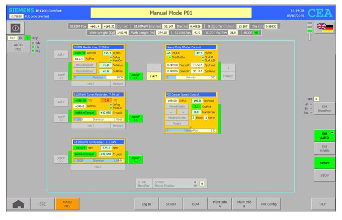
**Note:** in this very plant, the presented <u>S120M Master Line velocity</u> (ActVelo) you are seeing on HMI is the velocity on the motor shaft side and does not meet the load rotation. In other words, it is the velocity assigned to Winder Control – i.e. 42.3 m/min times <u>Gear Ratio</u>.
